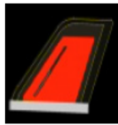
3d component of a blade antenna that is integrated into a large assembly, in this case, a helicopter.
